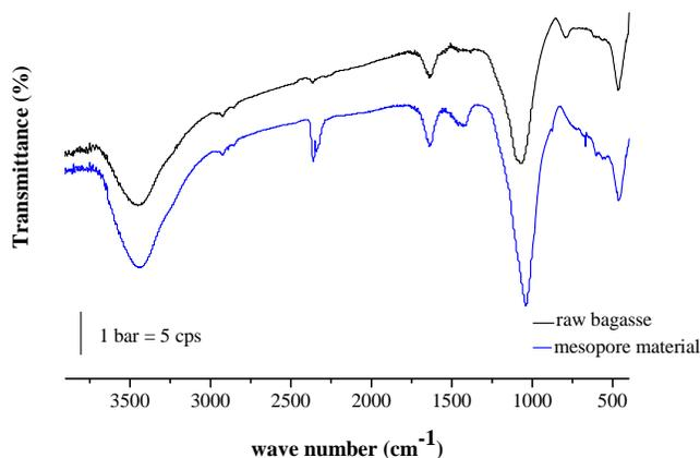
Figure 2. FTIR spectra of raw bagasse and mesopore material
