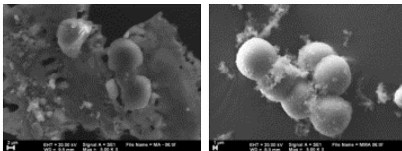
Figure 4. SEM images of bagasse unmodified CTAB (left side) and bagasse modified CTAB (right side)
