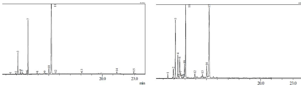
Figure 5. Chromatogram of initial patchouli oil (left side) and after adsorption process (right side)
