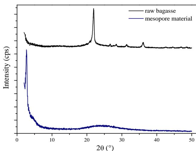
Figure 1. Diffractogram of raw bagasse and mesopore material
