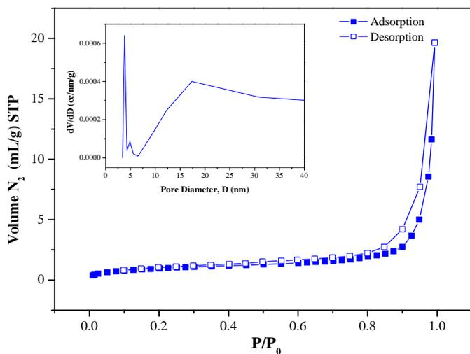
Figure 3. Nitrogen adsorption-desorption of mesopore modified bagasse
